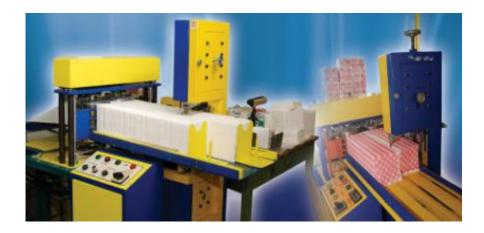
Machines for production of napkins, toilet paper, zig-zag towels, cores and cutter machine
